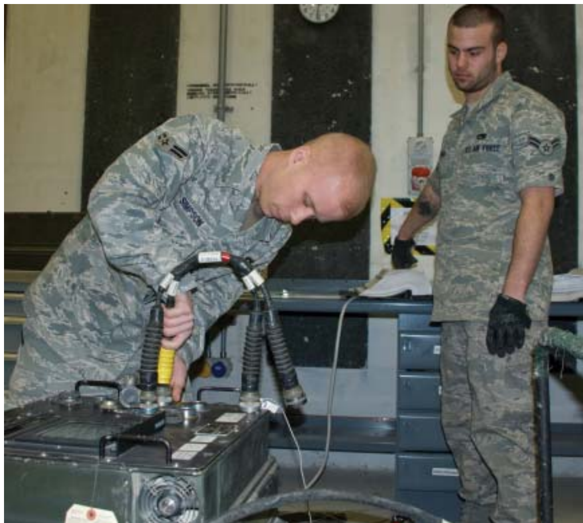
Airman 1st Class Kyle Simpson (left) and Airman 1st Class Jesse Camacho, both 31st MUNS precision maintenance specialists, prepare the guided missile test machine used to inspect ammunition.
